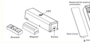
3. Use the screws or adhesive tape to fix the cover on the frame along the opening edge of the door or window. See figure below.
