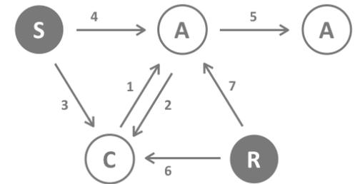
There are two different role a controller can have. There is always one single primary controller that is managing the network and including/excluding devices. The controller may have other functions - like control buttons - as well. All other controllers don't manage the network itself but can control other devices. They are called secondary controllers. The image also shows that its not possible to operate a sensor just from a remote control. Sensors only communicate with static controllers.
