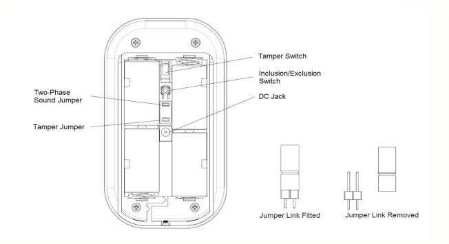
5. Use the rear cover as a mounting plate, mark the positions of the three fixing holes on the wall. Fasten the rear cover to the wall using the screws and wall plugs provided.
