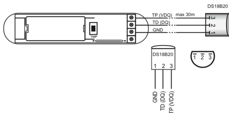
The external temperature sensor DS18B20 is connected to the device as shown in this picture. In case the sensor shall only act as temperature sensor it can be placed everywhere and there is no need to place the magnet nearby. Beside to act as temperature sensor the device can also work as simple digital sensor transmitting the status of an externally connected on/off switch. The subsequent image shows how to connect such an external switch to the pins 'IN' and 'GND'.
