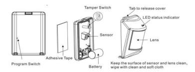
3. Using the adhesive tape to mount the device about 2 m above surface. To enhance operation place the device on a position which can detect the room widely. See figure below. The solid areas are the areas monitored.
