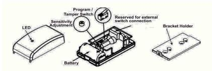
There are two options to mount the sensor. Double sides tape can be applied to the mounting plate or the device itself. Screws however offer a more solid mounting and are stongly recommended for all security-related applications.
